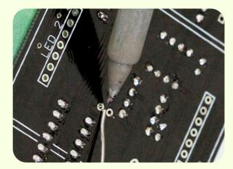
Fill the hole with solder. The legs on these are thinner. Make sure there is good contact.
