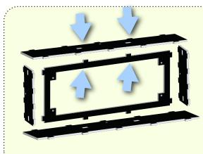
Once all the tabs are inside the holes, using only your fingers, pinch from the hole to the bottom of the tab, until each panel is as flush as possible with the PCB layer.
