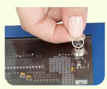
Finger tighten the DC barrel jack nut. Tighten as much as you can without using tools.
