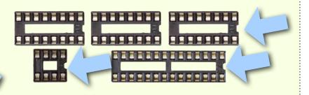
Hold each socket in place with tape, or carefully with your finger while soldering. Solder the first pin on one row, and then the last pin on the other row. Double check to make sure all of the legs are poking through, and the socket is laying as flat as possible on the PCB. If it's uneven, reheat the first and last legs while pressing the socket into place.
