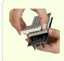
To mount the populated & tested PCB, you will need to remove the first LED module. Leaving the other three in place. Gently wiggle it out, trying as much as you can to not bend the pins on the modules.
