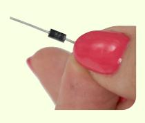
Grasp the diode a little bit away from the body, and bend the legs similar to the way you prepared the resistors.
