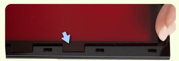
Peel the paper from both sides of the red filter, and place it 'into' the slots cut out to accept it on the structural front piece. Press firmly over the notched parts of the red filter, as well as around 1/8" tabs along the edge. The double sided tape will be holding the structural front, and red filter to the bezel.
