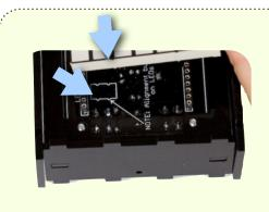
Flip the assembly over in your hand, so the LED modules are aiming up towards you, and support the PCB from the backside. With the PCB loose, you can carefully re-insert the first LED module. It goes in the same orientation as before. Mind the notches on the long sides.
