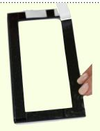
Remove the slippery white double-sided tape covering from one of the bezels
