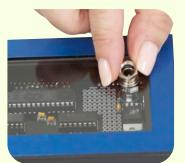
Take the remaining black screw, and finger tighten it through the hole into the rear structural layer.
