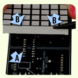
Hold the display along the short sides, pins down as in the photo (left). One side has 2 bumps, and the other side 2 recesses.
