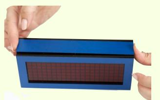
Very last step: Peel the blue protective covering. Start at one corner, and pull it away. Don't use a sharp object to get it started. A fingernail works best.
