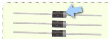
The Solder Time Desk Clock uses 3 of these diodes. Take a moment to notice that they have a grey stripe one one end. **These have polarity**, and can only be installed in one way.
