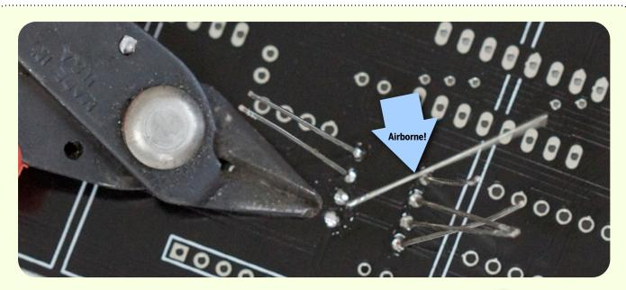
Carefully snip the excess legs. Use caution to not scratch the surface of the PCB.
