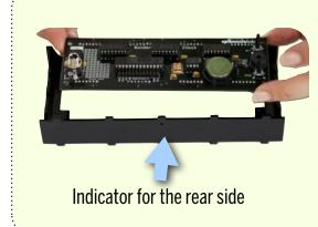
Place the structural housing with the indicator up. The PCB assembly gets installed from the rear side.
