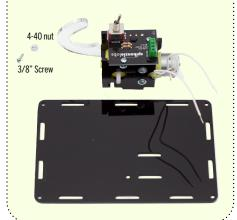
Line up the 2 slots, and place the motor assembly in place.
