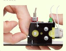
Tighten with a screwdriver, do not over tighten.
