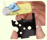
Place the arm side motor mount acrylic piece over the motor, making sure that the 'nub' fits in the hole in the mount.
