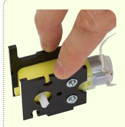
With the screws a little loose, press down against a flat surface, so that the both bottoms of the motor mount are flat.
