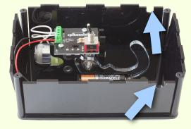
Place the acrylic rod that is glued to the bottom of the door into the hinge curves on the long sides.
