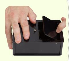
Once the top panel is set, take the washer, and place it over the toggle button. (Curved side up)
