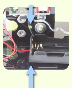
The right side has an equal distance between the arm and the slots along the left side of the bottom panel. Installed in this way, the battery holder is accessible, and will not interfere with the arm operation.
