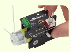
You will be using these nuts and screws to hold secure the PCB to the motor mount.
