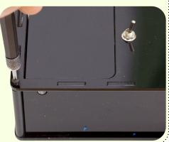
Only screw the top screws in until they touch the top piece of acrylic. If the corner posts are not flush, the top will flex. It is ideal to have the top piece laying flat.
