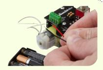
Touch the red and black wires to the wires connected to the motor. Pull one of the wires away and check the position of the motor shaft. Repeat until you have the motor shaft at a 12 o'clock position. Really close is good too.
