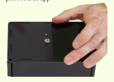
Screw the nut down, finger tight only. Do not use any tools for this.
