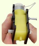
While holding the weld nuts in place, slide both screws through the washers, motor mount, motor and screw into the weld nut. For the moment, leave the screws loose enough so that the motor mount plastic can wiggle a little.
