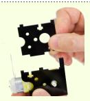
Hold the other motor mount as above. Place against the wire side of the motor
