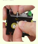
Using your fingers, tighten the screw. Make sure the nut does not slide out.
