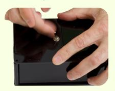
The remaining 4 black screws get sent through the holes in the corners of the top cover. Make sure that the screw and the round corner pieces are lining up as you go. Once again, do not over-tighten.
