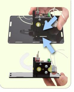
Slide the screw up through the bottom cover, and side the nut in so it rests in the slot.
