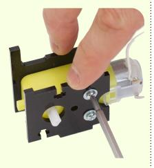
Keeping the bottoms of the motor mount flat against the surface, tighten both screws.
