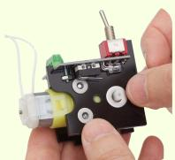
Align the arm piece so that the laser cut hole will fit the motor spindle. Press the arm over the spindle until the top of the spindle and the arm plastic are flush. The arm does not get pushed all the way down to the washer. Make sure not to bend the level on the snap switch with the arm, as you are attaching the arm to the motor spindle.
