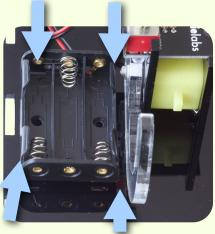
Peel the other side of the velcro backing, and attach the battery holder to the bottom panel.
