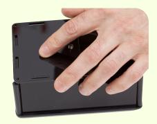
Move each of the side panels so that the tabs from all 4 sides are held within the slots on the top panel.
