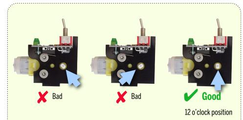
If your motor happens to be in the correct 12 o'clock position, skip to: **Attaching the arm**
