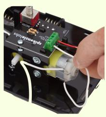
The top wire from the motor connects to the last screw terminal. Slide it in place, and screw it down.
