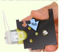
If the arm side motor mount is not fitting flush against the motor: Use a hobby knife to expand the hole in the motor mount.
