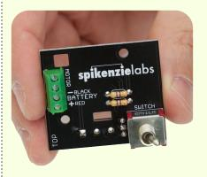
Place the PCB assembly over the motor assembly.
