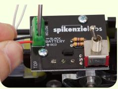
**Note:** Make sure to tighten the screw terminals onto the bare wire, and not the colored plastic casing. You may have to loosen the screw terminal in order to get the wire in.
