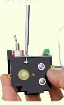
In the same way, slide in the other nut, on the other side, and attach the other screw.
