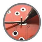
Touch solder to the pin and pad. (Not the iron) Solder should start to melt.
