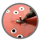
Allow solder to flow onto pin and pad. Remove solder. Count 2 seconds with the iron still touching.
