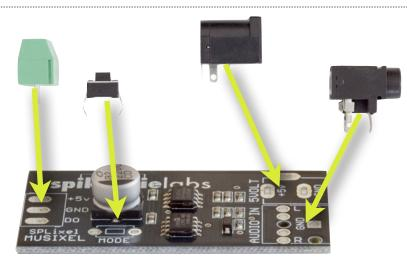
Place the parts onto the PCB. Make sure the openings point towards the outside of the board.
