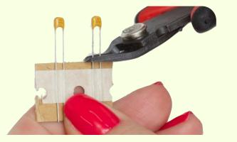
Place the capacitors in the two locations as seen in these photos. Marked as 0.1uf on the PCB.
