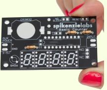
Flare out the legs to keep them in place. Be sure that the body of the resistor is flush against the PCB.
