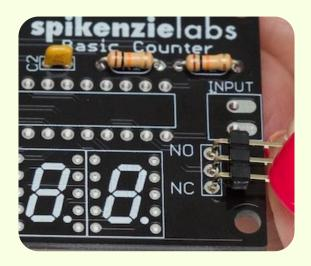
You can hold the pin header in place with a piece of masking tape. This makes it easier to solder.
