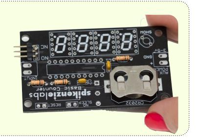
You can hold the clip in place with a piece of masking tape if you like. Solder the 2 pins.
