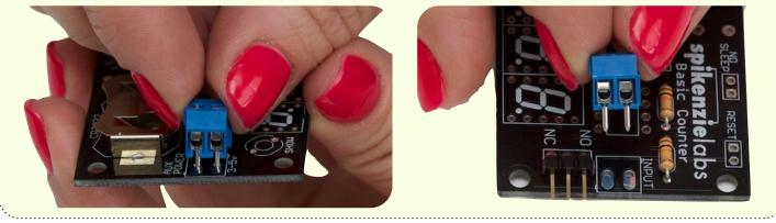
Solder both of the screw terminals in place. You can use a piece of masking tape to hold the terminals while soldering.
