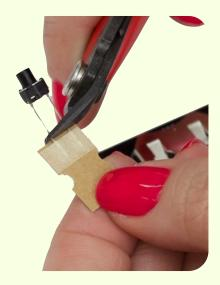
Slide the button through the 2 holes to the left of the LED displays.
