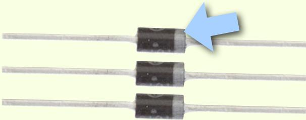
The Solder Time Desk Clock uses 3 of these diodes. Take a moment to notice that they have a grey stripe one end. **These have polarity**, and can only be installed in one way.
