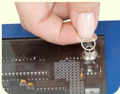
Finger tighten the DC barrel jack nut. Tighten as much as you can without using tools.
