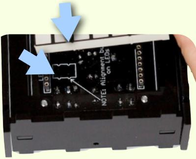
Flip the assembly over in your hand, so the LED modules are aiming up towards you, and support the PCB from the backside. With the PCB loose, you can carefully re-insert the first LED module. It goes in the same orientation as before. Mind the notches on the long sides.
