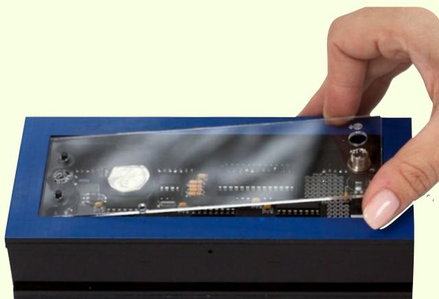
Place the DC barrel jack washer over the DC barrel jack.
