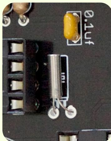
Spread the legs, and insert one of the crystal legs into each hole
