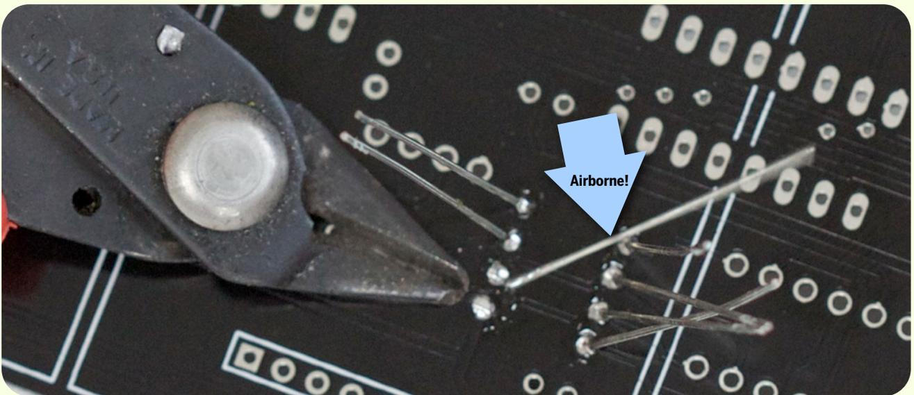
Carefully snip the excess legs. Use caution to not scratch the surface of the PCB.
