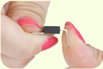
Place it onto the PCB, the three legs through the holes, and the metal back plate touching the exposed metal pad on the PCB. Tape in place.
