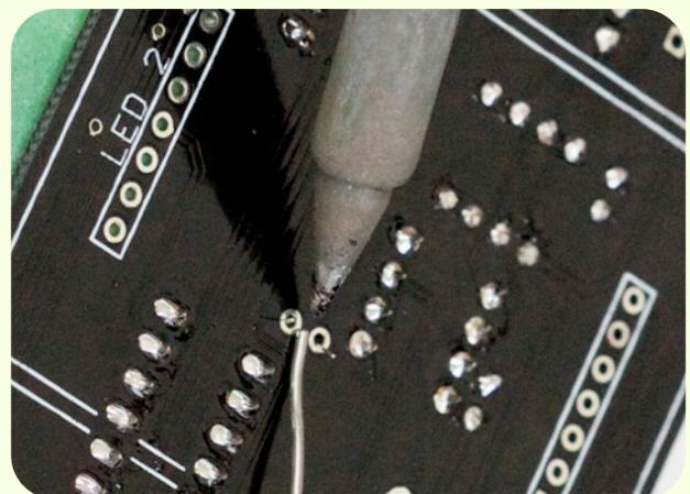
Fill the hole with solder. The legs on these are thinner. Make sure there is good contact.
