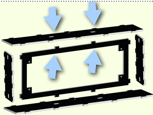
Once all the tabs are inside the holes, using only your fingers, pinch from the hole to the bottom of the tab, until each panel is as flush as possible with the PCB layer.
