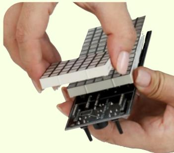
To mount the populated & tested PCB, you will need to remove the first LED module. Leaving the other three in place. Gently wiggle it out, trying as much as you can to not bend the pins on the modules.
