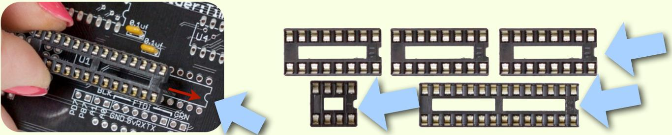
Hold each socket in place with tape, or carefully with your finger while soldering. Solder the first pin on one row, and then the last pin on the other row. Double check to make sure all of the legs are poking through, and the socket is laying as flat as possible on the PCB. If it's uneven, reheat the first and last legs while pressing the socket into place.
