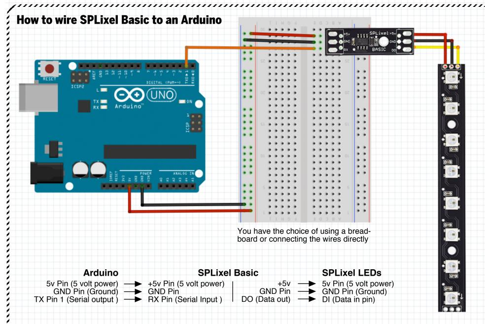
NOTE: Only use this hook up method for 1 to 16 LEDs strips. This type of WS2812 LED draws lots of power, so we do not recommend connecting longer strips directly to the Arduino as the Arduino's voltage regulator may not be rated for the amps required. For longer strips up to 64 LEDs, see our guide for connecting long strips to the SPLixel Basic.
